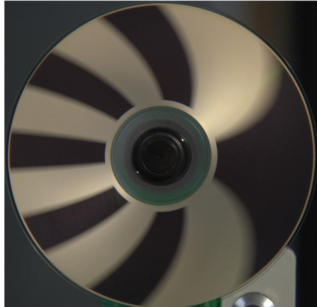
**Figure 6 Rotating fan, rolling shutter at 1/1000**
