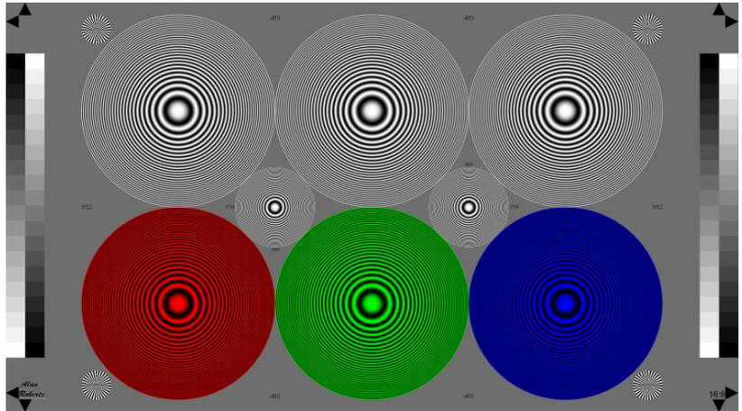
Figure 1, zone plate test chart
