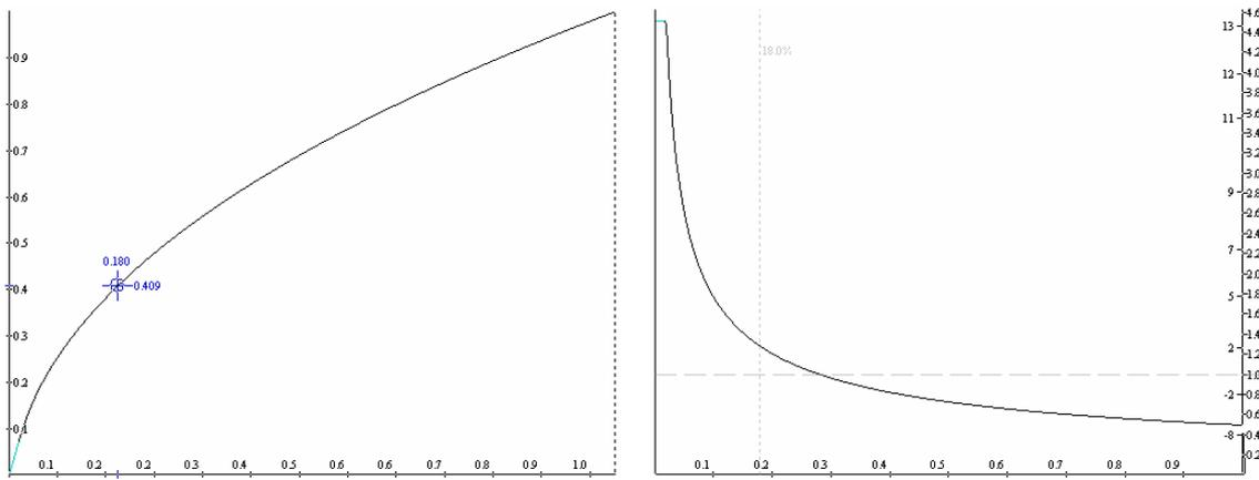
Noise performance usually follows the slope of the gamma curve, since noise is generated mostly in the analogue front end of the camera. Although the gamma curve selected in the camera was called “CCIR” it is probably intended to be that of ITU.R-BT 709 (left-hand plot).
