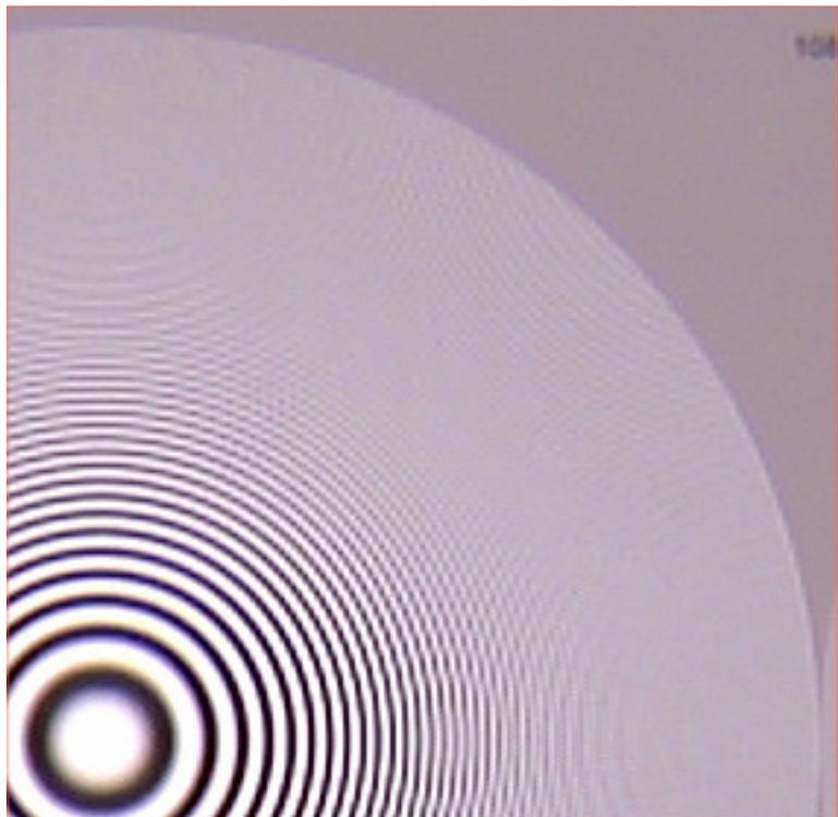
The aliasing is not particularly strong, indicating that either there is probably good optical low-pass filtering (bi-refringent). The diagonal aliasing from the quincunx precision offset is well suppressed
