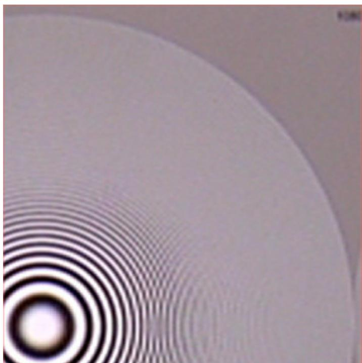
the down-conversion is correctly limiting the vertical to that admissible in an interlaced signal. However, since the HDTV image is not particularly sharp anyway and relatively free from aliasing, the down-conversion is actually rather good.
